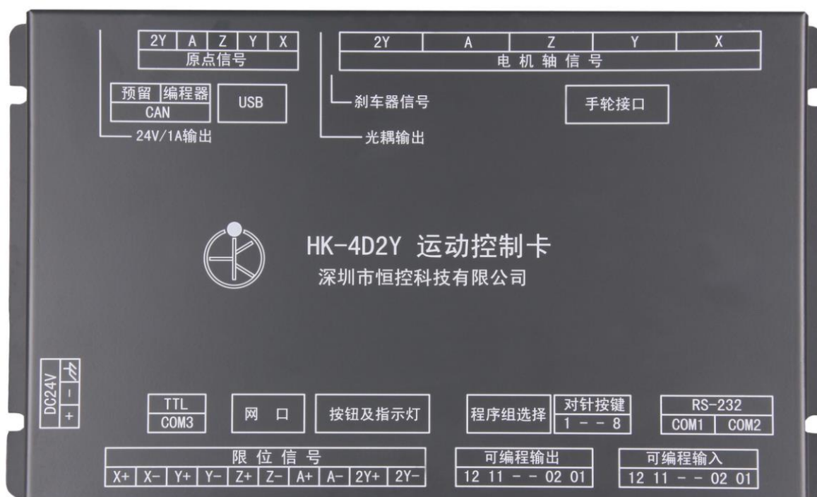
HK- 4D2Y Main board (224mm * 130mm * 42mm)
