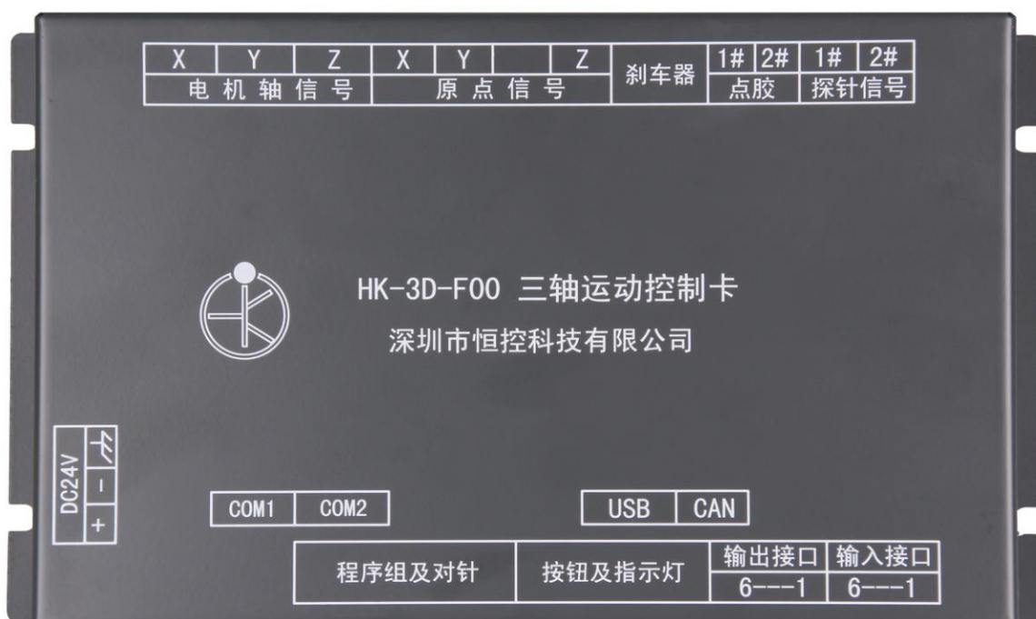
HK-3D-F00 Main board (194mm * 110mm * 42mm)
